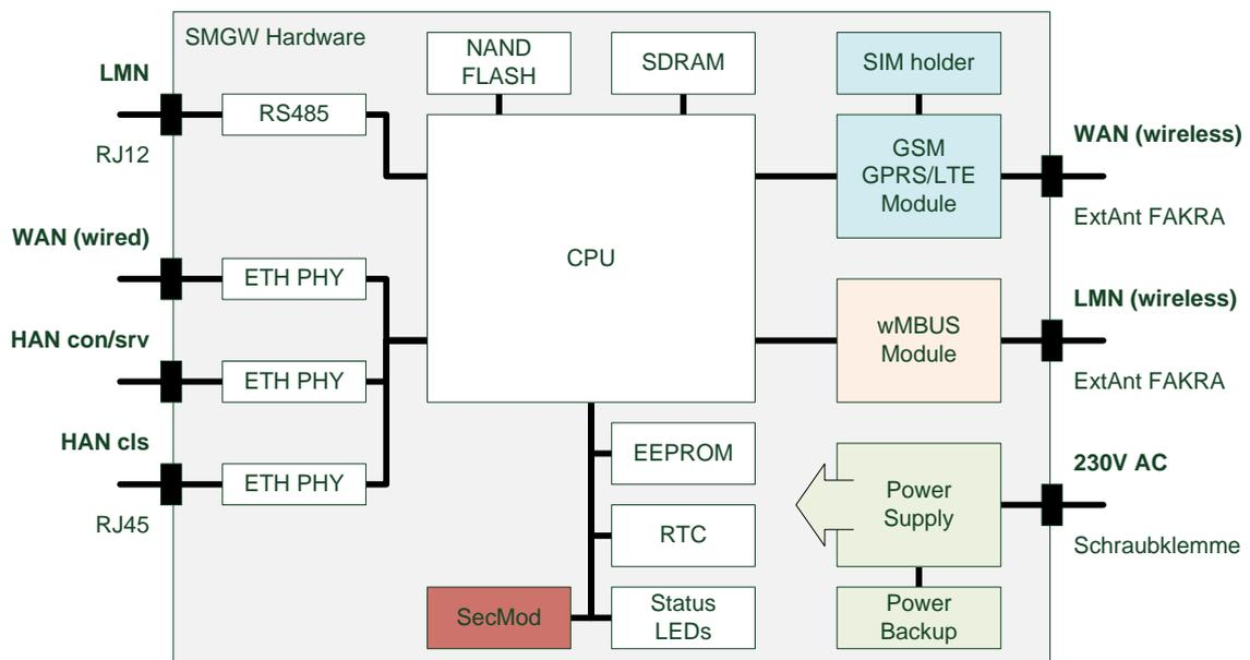
Figure 4: SMARTY IQ-SMGW internal structure
