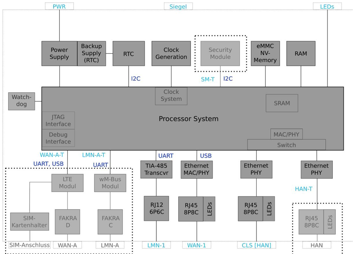
Figure 1.6: The hardware parts of the TOE
