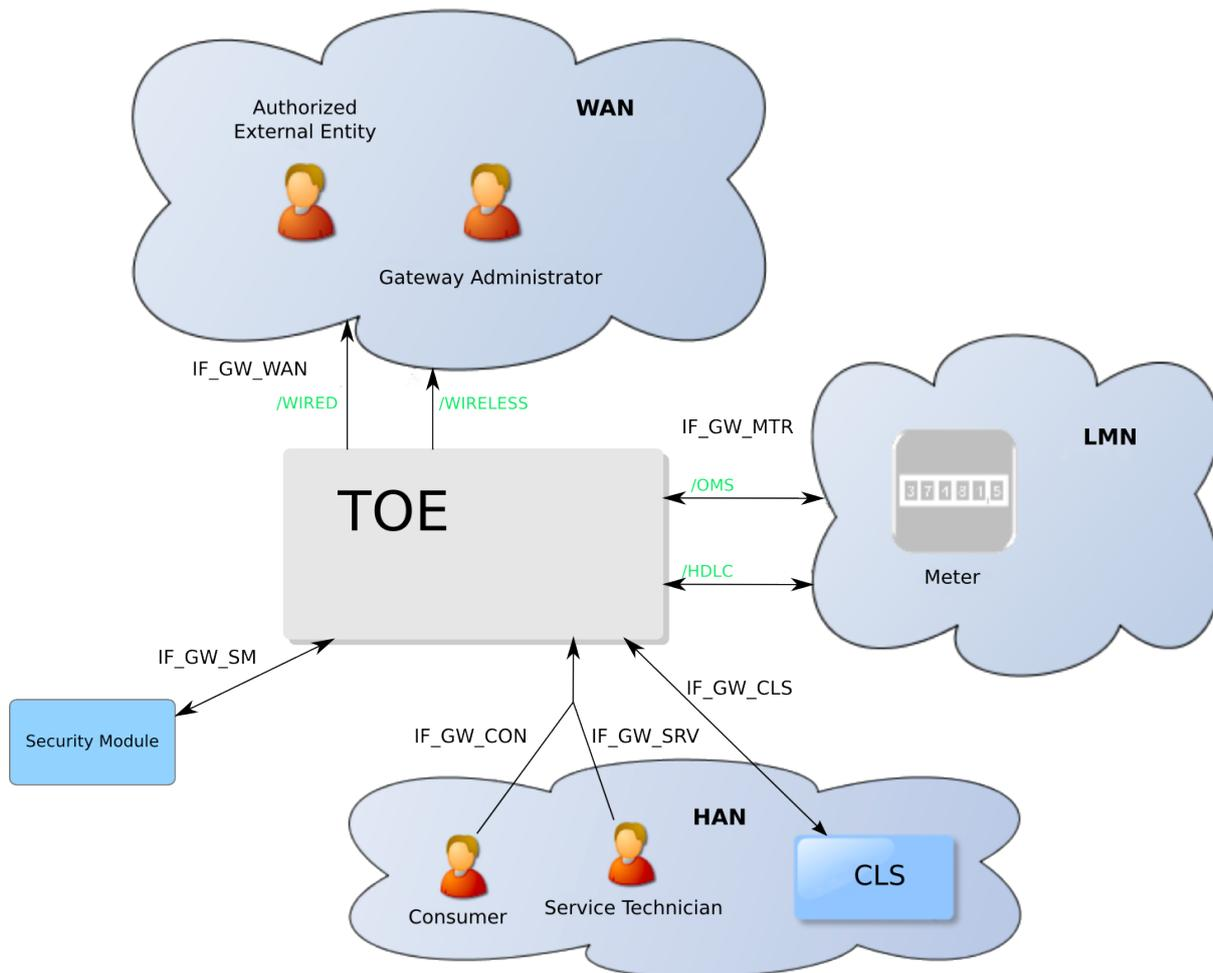
Figure 1.2: The logical interfaces of the TOE
