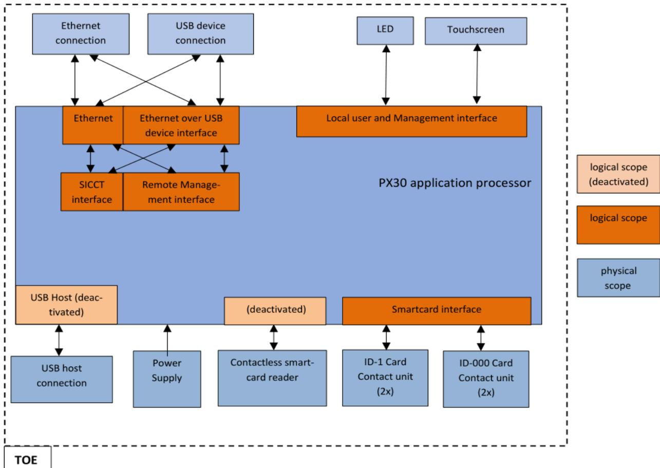
Figure 1: TOE Architecture
