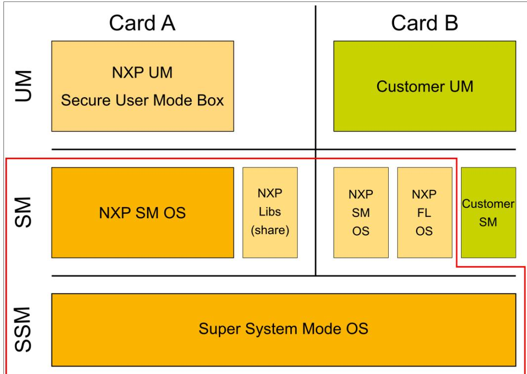
Figure 3. Software components of the TOE
