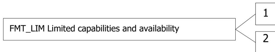
FMT\_LIM.1 Limited capabilities requires that the TSF is built to provide only the capabilities (perform action, gather information) necessary for its genuine purpose.
