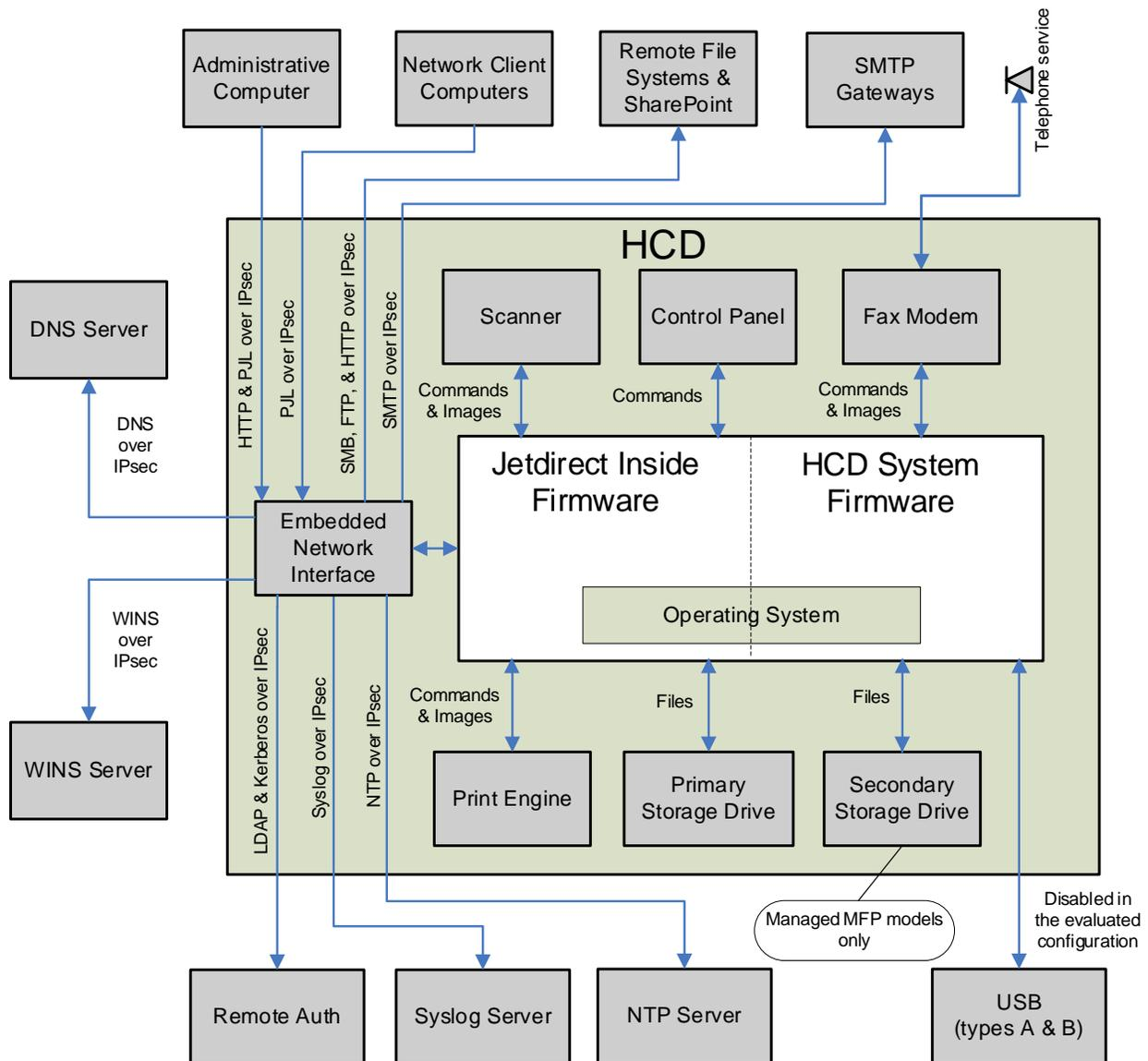
Figure 1 shows a high-level physical diagram of an HCD with the unshaded areas representing the TOE and the shaded areas indicating components that are part of the Operational Environment.
