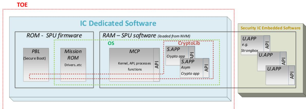
Figure 2: TOE software design decomposition
