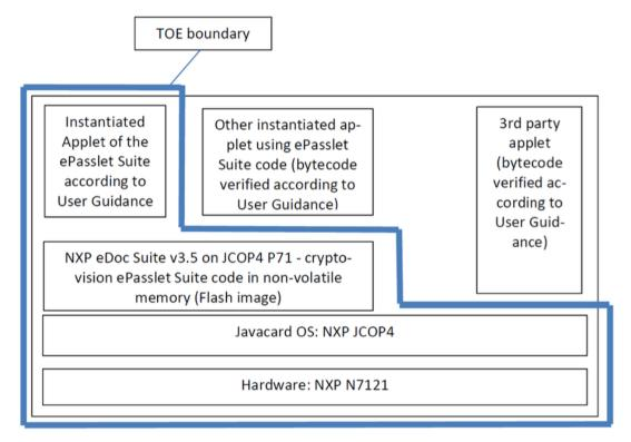
Multiple configurations (and hence support for different applications) can be present at the same time by instantiating multiple applets with their distinct configurations. Such additional functionality is independent of the functionality of the TOE as described in the [ST] and the guidance manuals. This is ensured by the isolation properties of the Java Card platform.
