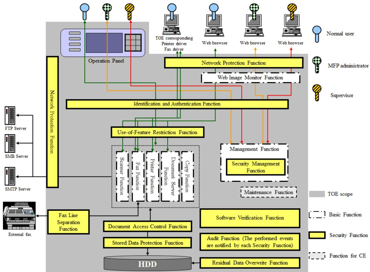
Figure 5-1 TOE Components
