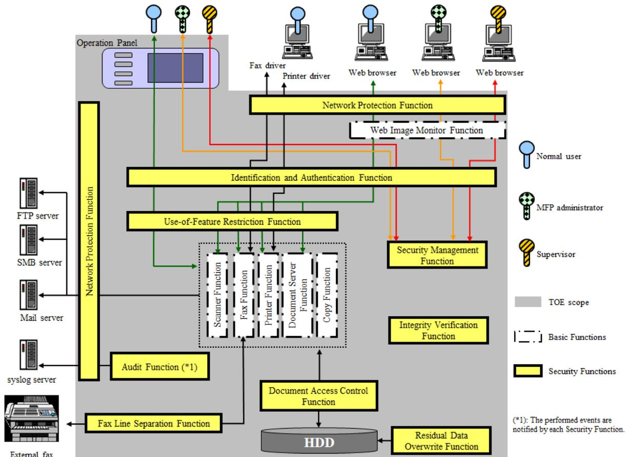
Figure 5-1 TOE Components
