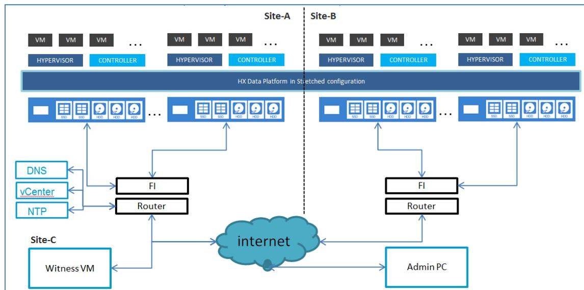
Figure 2 TOE test configuration overview (Site A, Site-B, and Site-C are located in the same location).
