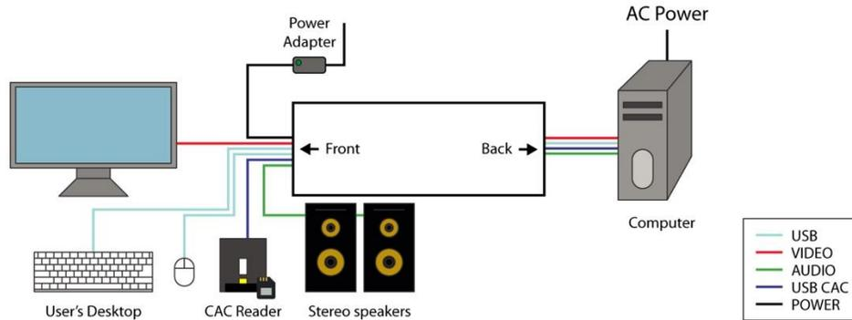
Figure 1: Standard Setup of 1-Port KVM TOE Installation
